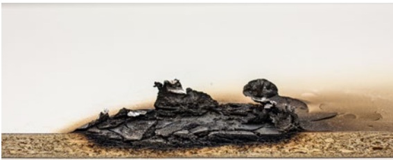
Cross-section Decorative Flammex Particleboard after 30 minutes of burning
