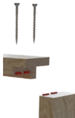
Trenched or Half Lapped Joint
