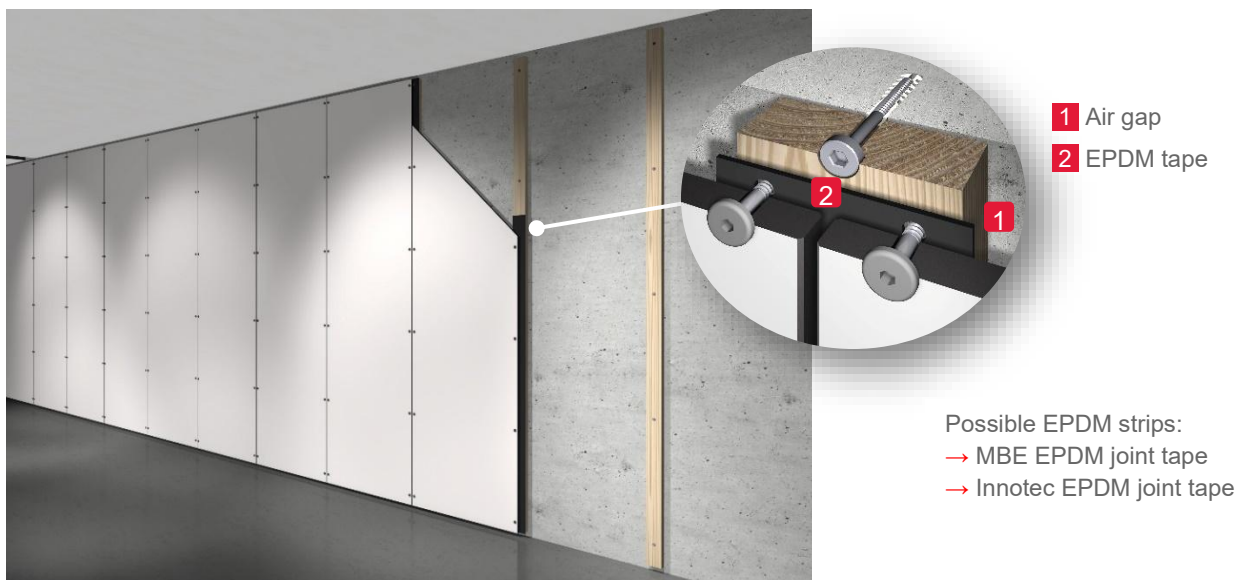
Figure 25: Visible mechanical fastening
