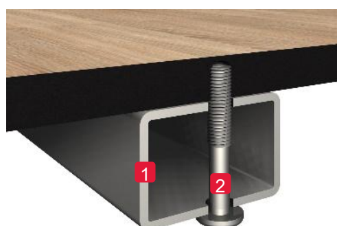
Figure 41: Recommended fastening method for the compact tabletop
