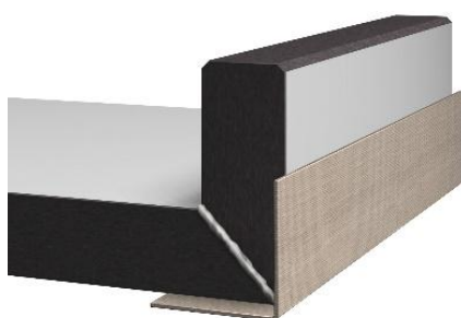
Figure 18: Fold up the upstand and secure it with adhesive tape
