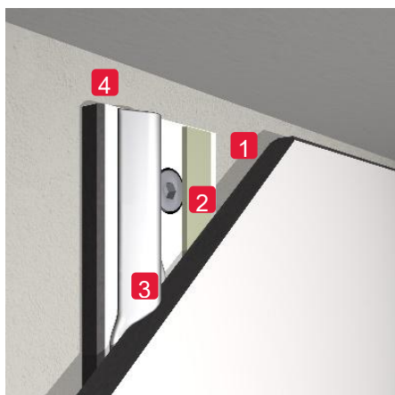
Figure 30: Finishing the wall cladding at the top
