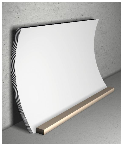
Figure 3: Incorrect storage of Compact Laminates
