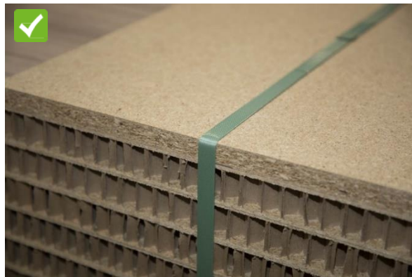
Always secure consignment packages with two PVC straps and ensure that 16 - 19 mm protection boards - top and bottom - are used for each new package.
