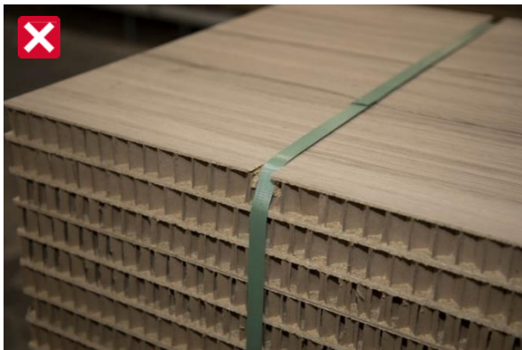
Damage when using PVC straps without protection board.
